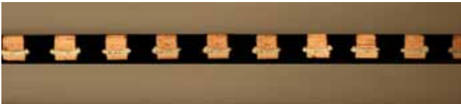
Thermal Compression bonded (TCB) micro-bumps on the TSV tips in fcFBGA
